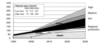
Figure 8.8 Natural gas demand of Northeast Asia, 1990–2030 (million tons per annum of LNG equivalent)
