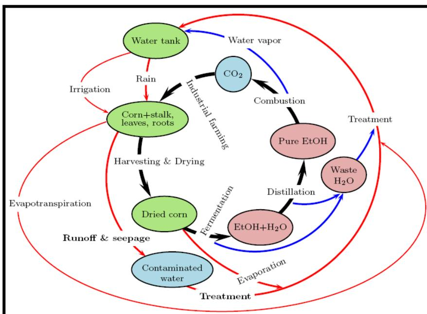
Diagram 9 - All inputs and outputs for ethanol production.
