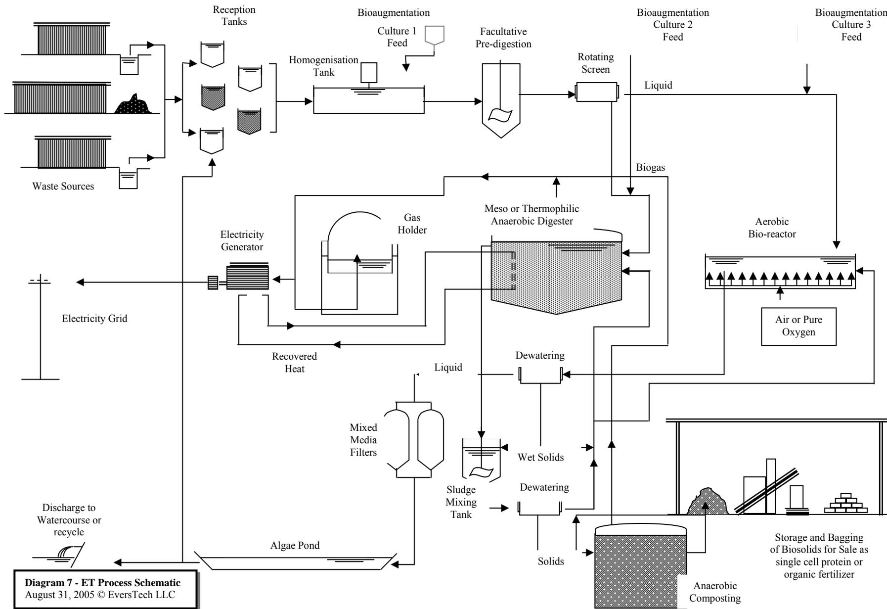
**Diagram 7 - ET Process Schematic**
